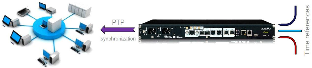
**Figure 2** Clock synchronizing a network by means of PTP.
