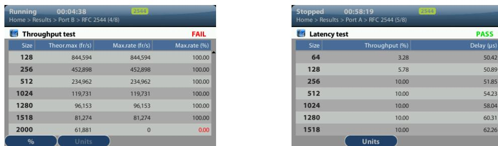
Figure 3 RFC 2544 test results: (a) Throughput results table, (b) Latency results table.
