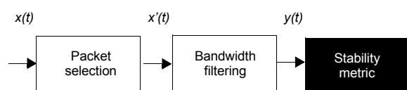
Figure 16 ITU-T G.8260 pkfilteredMTIE and pkfilteredTDEV preprocessing.
