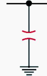
Lightning arrester (valve type)
