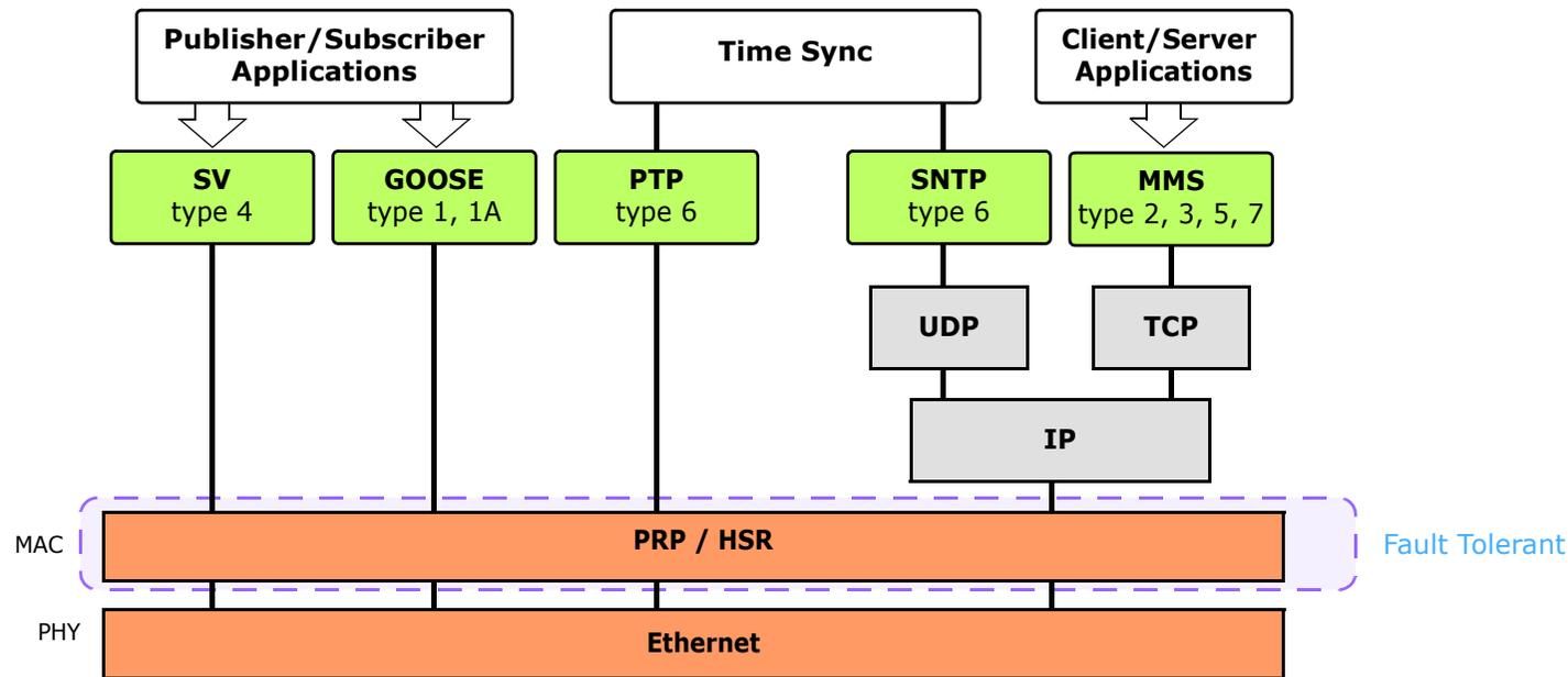
Network redundancy is crucial for maintaining **high network availability**, and many redundancy technologies can provide millisecond-level recovery. However, some mission-critical and time-sensitive applications **cannot tolerate** even a **millisecond** of network interruption without severely affecting operations or jeopardizing the safety of on-site personnel.
