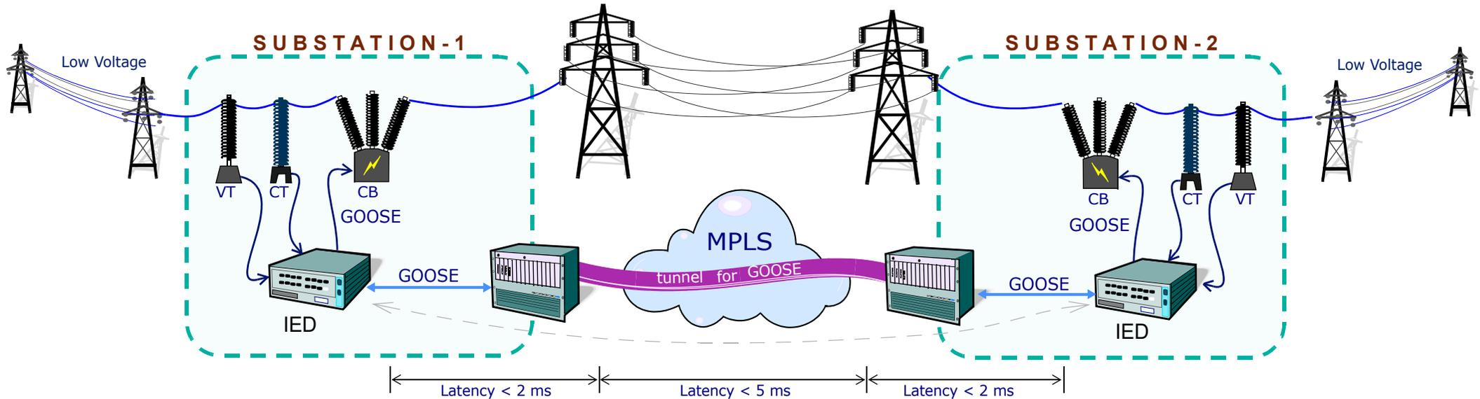
GOOSE is a Layer 2 protocol (not routable) used by IEDs send messages inside the substation LANs, nevertheless using MLPS it can be extended to remote substations and Tele-protection. MPLS facilitates GOOSE traffic through the WAN extending the LAN thus IEDs can exchange information with remote devices at remote substations:
