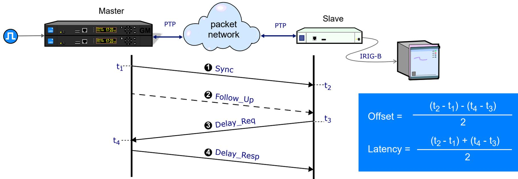
It is a cost-efficient solution and can be applied on the basis of the existing Ethernet network in a substation. PTP (IEEE 1588) applies master/slave time synchronization mechanisms and supports hardware time stamps. The basic parameters of Latency / Offset are computed from the  $t_{1...4}$  stamps.
