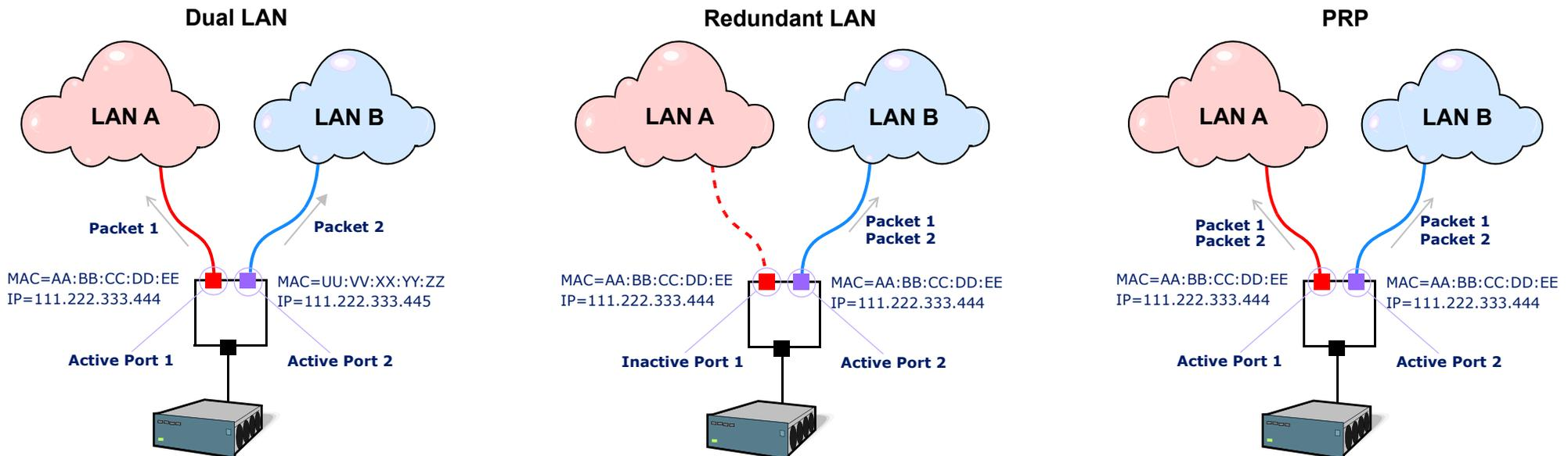
PRP is based on the use of two independent networks: LAN A & LAN B
