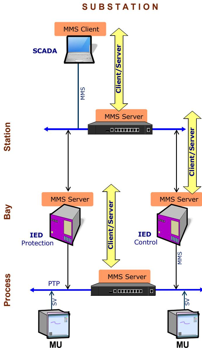
MMS is used by the applications to **transfer data** between substation levels, communicating IEDs and SCADA systems to move the information such as device status, obtain reports, data acquisition in order to monitor and get control.
