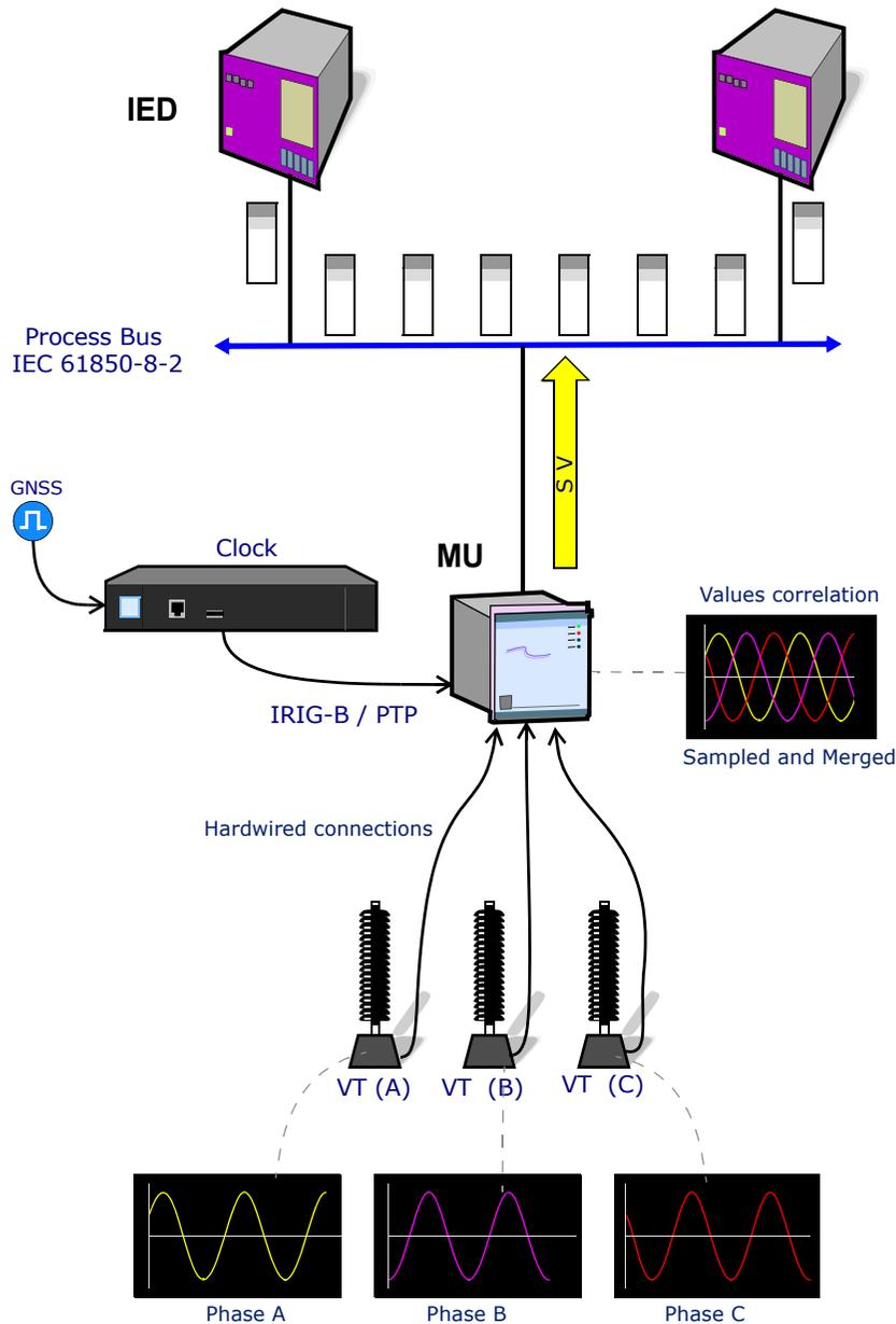
A **Merging Unit (MU)** is an IED that digitizes the analog measurements taken by current and voltage transformers. Afterwards the MU publishes the data as a stream at a predefined rate.
