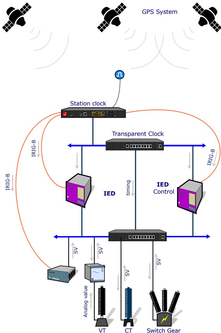
Many Utilities acquire timing from GNSS and the station clock converts signal into a 1-pps or IRIG-B code, which are then distributed by dedicated links to all the IEDs in a substation. However, important to say that this system has some **weaknesses** (\*) being **vulnerable** to human and natural disruptions that may perturb normal operations by raising false alarms, delaying actions, and lowering system efficiency.
