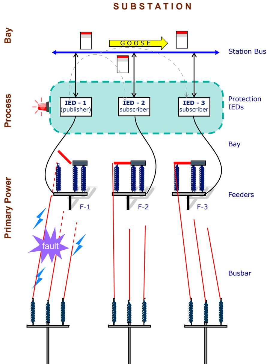
A fault causes a voltage drop on a feeder and, after the clearing of the fault, results in an inrush condition (a sudden arrival of energy) which may lead to an undesired operation of protection on the healthy feeders.
