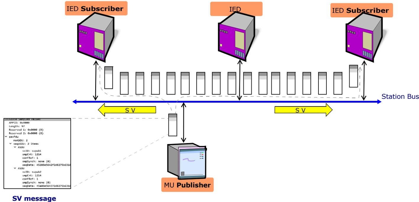
It is defined in the standard to provide a fast and cyclic transfer of samples.
