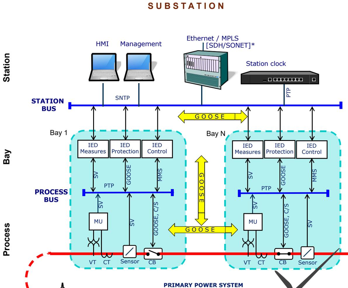
GOOSE most often applications is used for **protection, control and automation** of electric systems.
