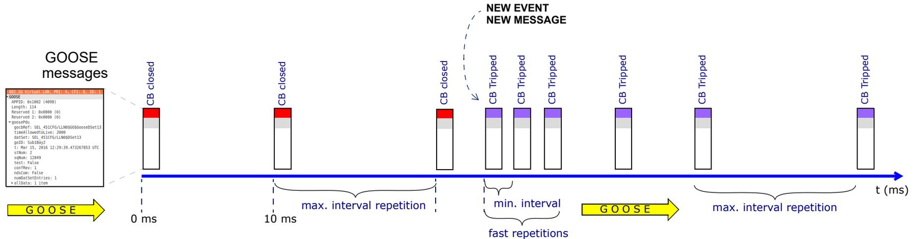
Since the GOOSE messages replace hard-wired signals used for protection and control applications IEC 61850 introduces mechanisms that ensure the delivery of the required information.
