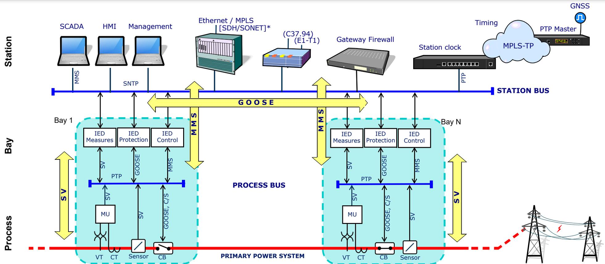
The **Station bus** provides connectivity to individual bays, distributed controllers, gateways, management and human machine interfaces (HMIs). It may connect up to hundreds of Intelligent End Device (IEDs), often segmented physically or logically depending on their application.
