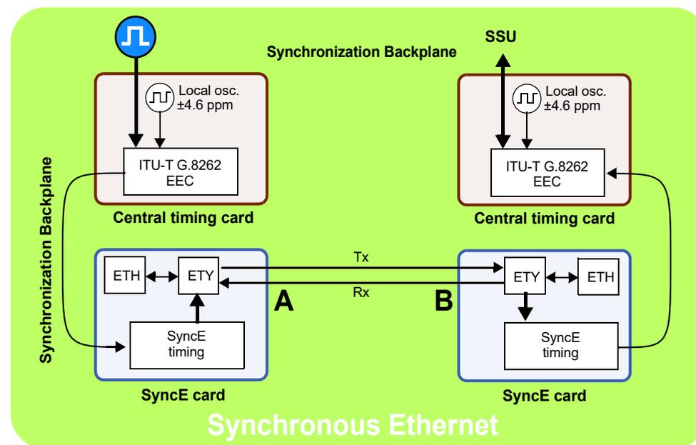
SyncE is not part of the IEC 61850 but is being used in the Power industry
