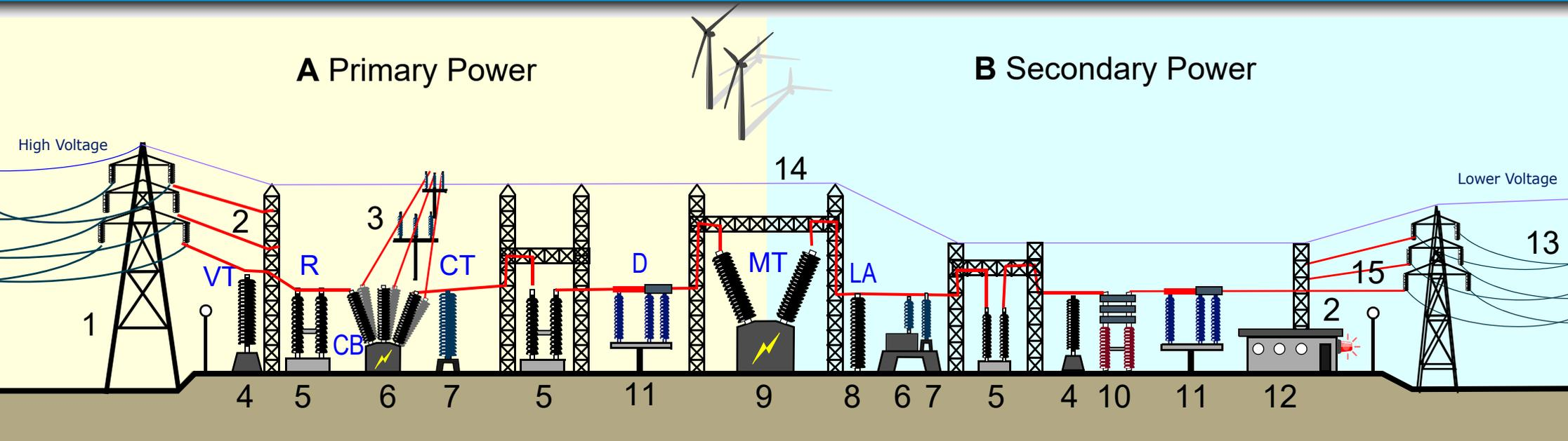
1.Primary Power (PP), 2.Feeder, 3. Busbar, 4.Voltage Transformer (VT), 5.Relay (R), 6.Circuit Breaker (CB), 7.Current Transformer (CT), 8.Lightning Arrester (LA), 9.Main Transformer (MT), 10. Capacitors (C), 11.Disconnector, 12.Control Shelter, 13.Secondary Lines, 14. Ground, 15. Overhead Lines
