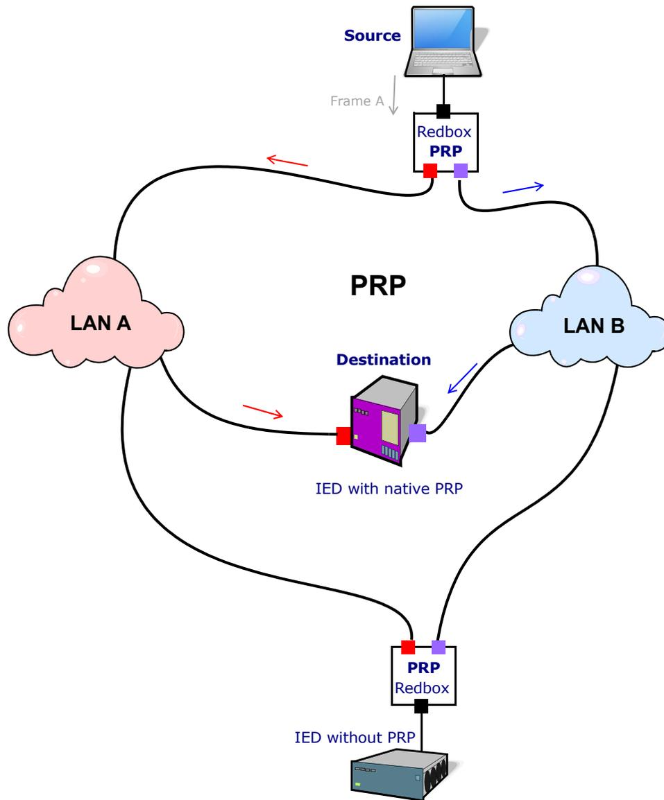
Network redundancy is crucial for maintaining **high network availability**, and many redundancy technologies can provide millisecond-level recovery. However, some mission-critical and time-sensitive applications **cannot tolerate** even a **millisecond** of network interruption without severely affecting operations or jeopardizing the safety of on-site personnel.
