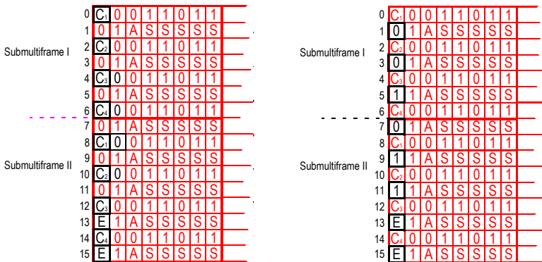
Figure 1.6 The CRC-4 provides error monitoring by means of four C i bits that correspond to the previous submultiframe. If the receiver detects errors, it sets the E-bit to indicate the error. The “001011” sequence is used to synchronize the submultiframe.
