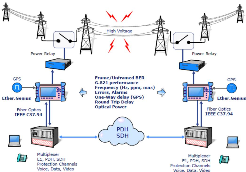
Fiber optics do not need ground and are immune to the interferences caused by electrical noise therefore eliminates a lot of the errors that electrical connections do suffer. In other words, it is convenient the use of fully optical links from power relays to Multiplexers as the IEEE C37.94 standard defines.
