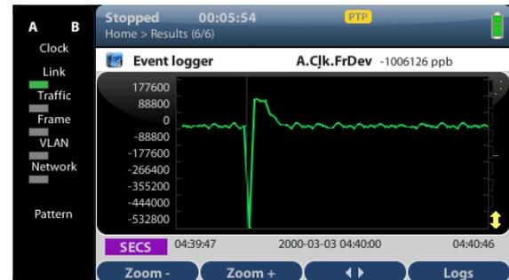
ALBEDO Ether.Genius is a multi-technology tester equipped with all the features you need to install or maintain telecom networks based on Gigabit Ethernet (GbE), Synchronous Ethernet (SyncE), E1, Datacom, Precision Time Protocol (PTP IEEE 1588), Jitter/Wander, C37.94 and One-way-delay test.
