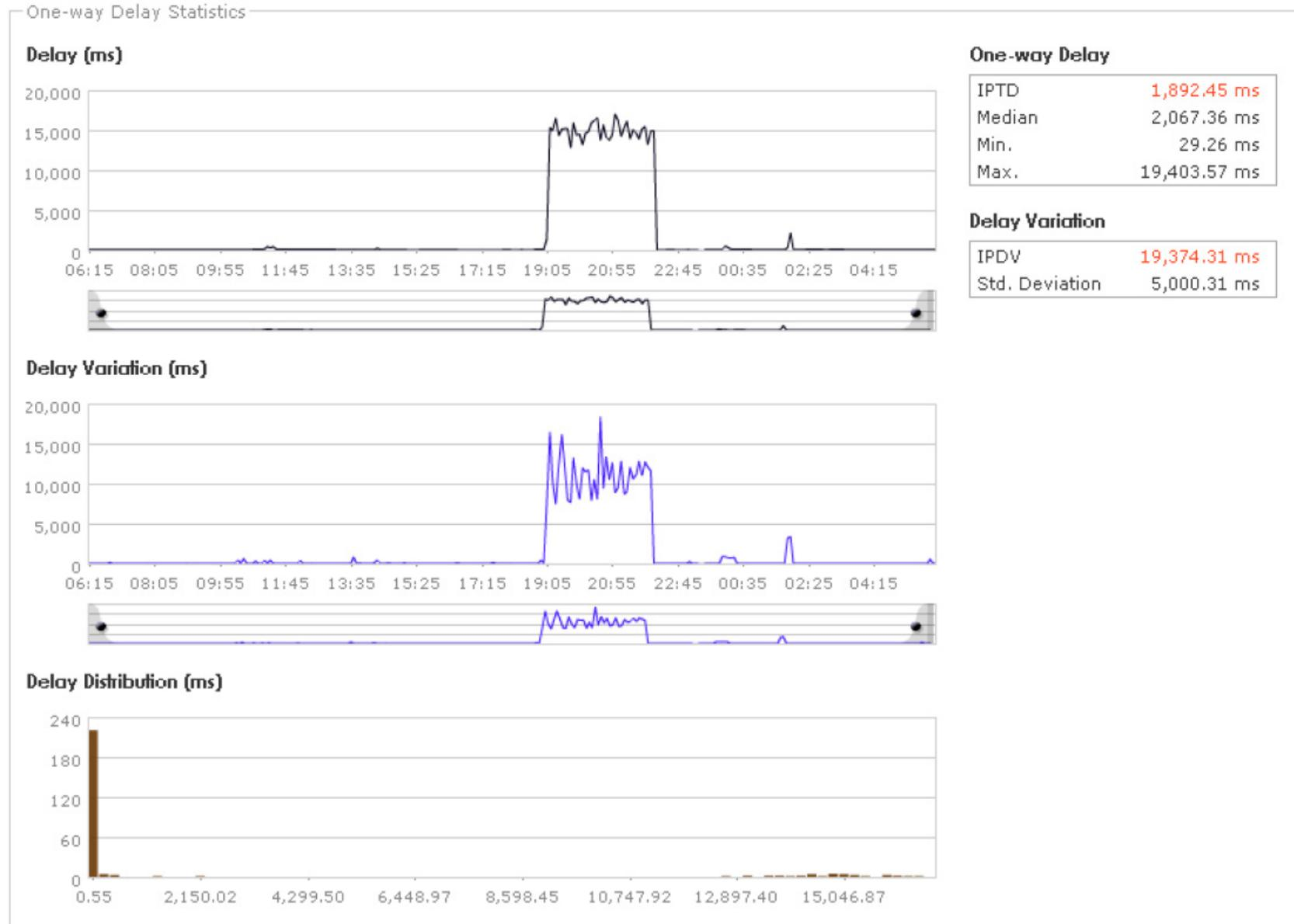
IP Networks require ONE-WAY-DELAY measurements because UP/DOWN delay is often different
