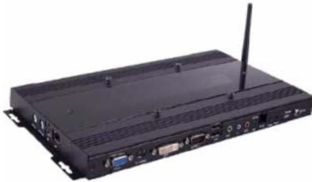
This probe checks compliance of [SLA agreement](#). Predicts the ability of a Carrier-grade Ethernet / IP network to support Multiplay services - Determines the ITU-T [quality of service](#) and analyses potential degradation sources - Meets ITU-T and IETF test standards. Synchronization through [NTP, GPS or atomic clock](#). Web/Internet user interface - It does not interfere with the monitored services - Secure data transmission and storage preserves privacy in monitored systems.
