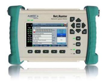
Both capture, forward & save packets in real time without generating jitter, delays or loss. Net.Hunter is a stream-to-disk device that can capture packets without disturbing live traffic
