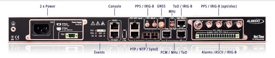
Net.Time simplifies the transition to PTP providing seamless translation between all the protocols installed in the Substations including NTP, PTP, SyncE, ToD or IRIG-B to PTP and viceversa. Equipped with a Rubidium or OCXO oscillator, Net.Time supports the widest variety of time references and distribution signals in order to simplify the synchronization of new and legacy appliances.
