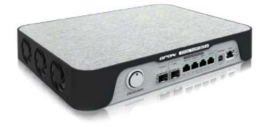
GPON Doctor OLTe has been designed primarily for ONT/ONU conformance and network interoperability testing, the GPONDoctor OLT-e is a perfect tool for lab application engineers involved in the GPON pre-deployment phase, as well as GPON network element vendors.
