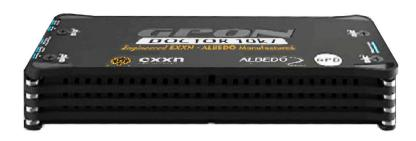
GPONDoctor 10K7 is a GPON + XGSPON protocol analyzer that captures up-downstream data, interprets PLOAM and OMCI level control information, extracts user traffic at the Ethernet layer, measures optical power, detects and reports line faults.
