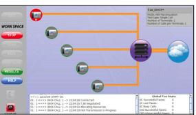
T.38 Fax emulation allows the VoIP network to be tested for its ability to successfully transmit and receive Fax over IP.
