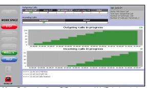
Mass Call mode allows SIP trunks and VoIP devices to be tested for call capacity under outgoing and incoming calls.
