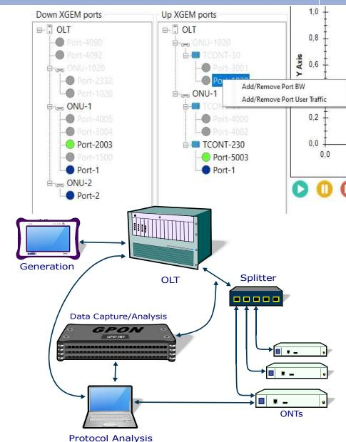
Fig 3. GPON Doctor 9k7 in operation, a xGenius as traffic generator and a Labtop for offline analysis.
