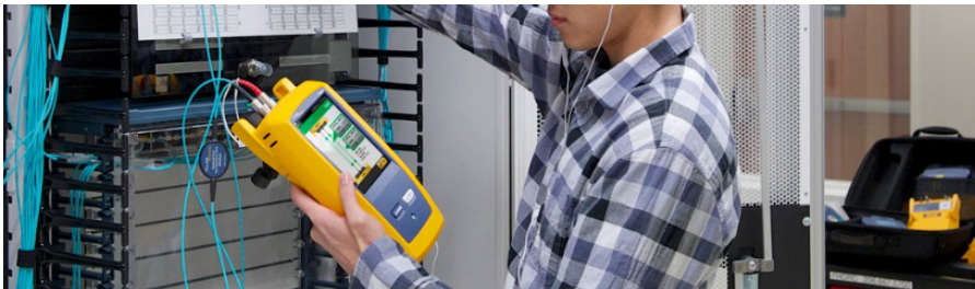
Figure 10.12 LANTEK 7 cable tester compliant with Categories 3/5e/6 and 7/ISO F standards, with a frequency range up to 750 MHz.
