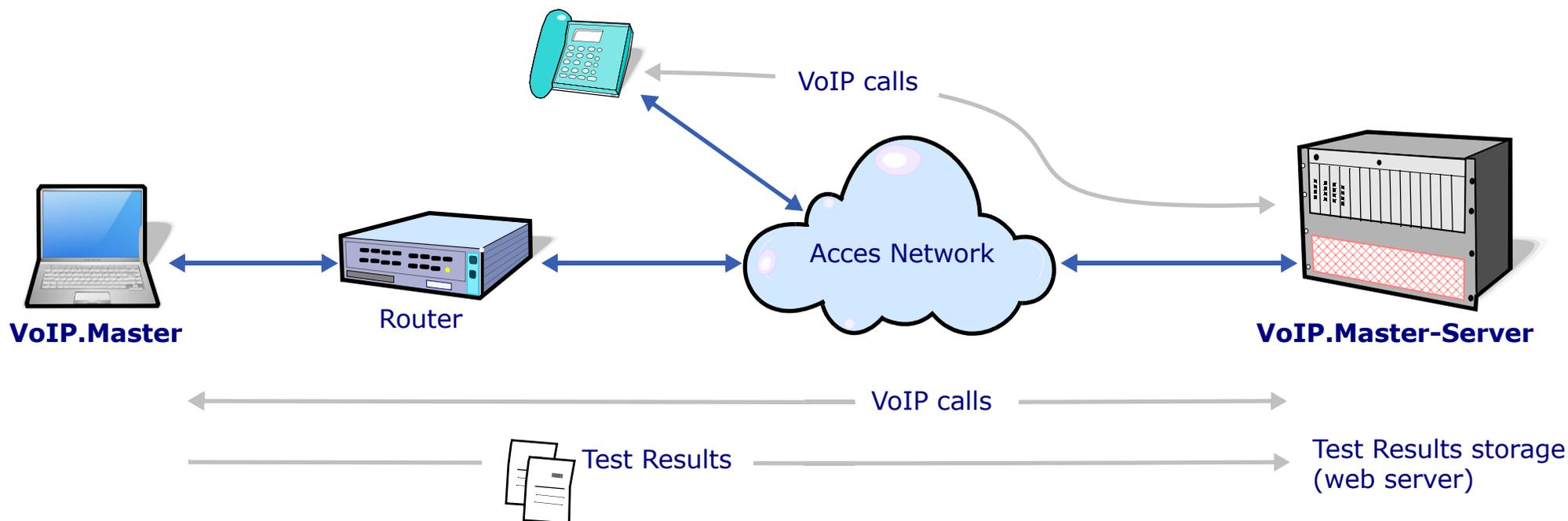
This is **centralized version** which is based on a Server that can work with VoIP.Master or directly with VoIP terminals to improve test process and increase technician efficiency and productivity:
