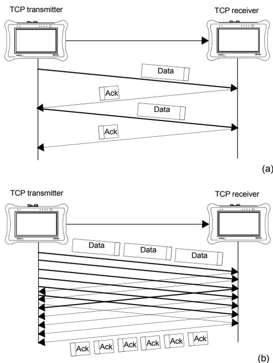
**Figure 1.1:** (a) No window is used: The transmitter has to wait for the acknowledge message to resume transmission. (b) TCP window mechanism: Continuous transmission can be achieved.
