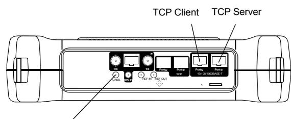
**Figure 2** Albedo xGenius test and clock reference interfaces used in this testing scenario.
