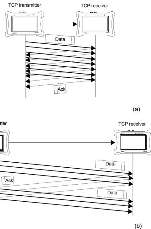
**Figure 1.2:** The importance of setting a correct window to achieve optimum performance in TCP data transfer: (a) The window is set to a value larger than the BDP and transmission is continuous. (b) If the window is smaller than the BDP the transmitter has to stop at some points and wait for acknowledge messages from the far end.
